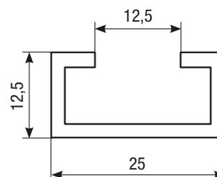
Type "SAL25" | "L"-shaped profile | for edges type B1NC-AG
